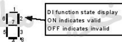
Figure 6-36 Definition of 7-segment LED
